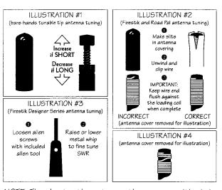
NOTE: The shorter the antenna, the more sensitive it is to adjustments. For example, two turns on a 4 foot antenna might move the SWR by 0.3; the same amount on a 2 foot antenna may move the SWR by 1.0. Make smaller adjustments on shorter antennas.
