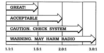
If measurements are below 2.0 to 1 on both channels, it isn't necessary to make any adjustments unless you want to fine tune the system to balance the SWR at both ends of the band. However, keep in mind that if SWR, regardless of the reading, is the same on channel 1 and 40, adjustments to the antenna may have a negative effect.
