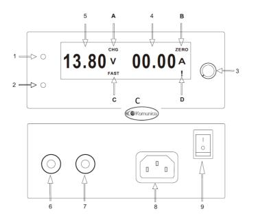
**1 Power indicator**: Light up when the unit turn on. **2 Warning indicator**: Light up when output terminal short or overload, over voltage (preset 16Dcv), component over hot.
