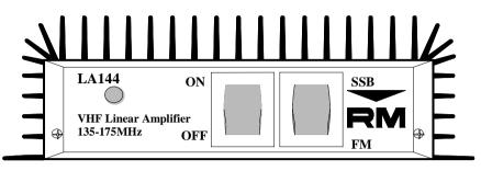
The LA144 is a wideband compact amplifier for the VHF band; covering from 135 to 175 Mhz. Output is nominal 60W at full power (70W max).
