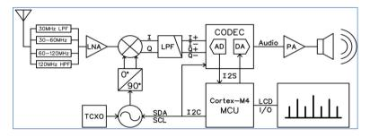
The clock generator Si5351 generates two quadrature square wave signals with variable frequency as they are excited it creates an ultra-low noise ZIF zero-IF receiver. The IQ signal obtained after mixing is output to the CODEC and collected by the MCU, and the DSP algorithm in the MCU, this completes the demodulation and display of the signal.
