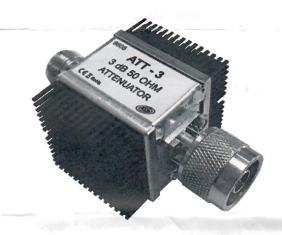
The ATT-3 attenuator is designed to reduce the RF signal by approximately 3.2 dB with a maximum input power of 10 W in the frequency range from DC to 500 MHz.
