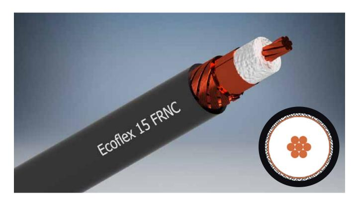
Ecoflex 15 FRNC is a flexible low loss 50 ohm coaxial cable for the frequency range up to 6 GHz. Advanced manufacturing techniques combined with the use of a low loss PE-LLC dielectric with a foaming rate of more than 70% result in very low attenuation values.
