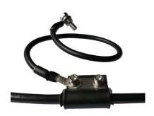
The GC-15 grounding clamp was developed for equipotential bonding on 15 mm coax cables such as ECOFLEX 15 etc. This eliminates potential differences (voltages) between the coax cable and the earth potential. Especially during thunderstorms, charging can occur on the antenna or on the coax cable. This charge is removed with the earthing clamp and the connected device is protected. A grounding clamp is not a replacement for lightning protection.
